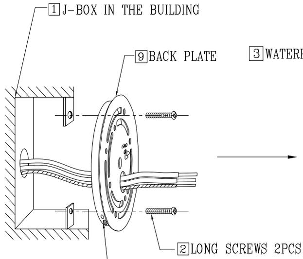
WHEN INSTALL THE FIXTURE, THE THREAD HOLE ON SIDE EDGE OF BACK PLATE SHOULD BE DOWNWARD VERTICALLY.
